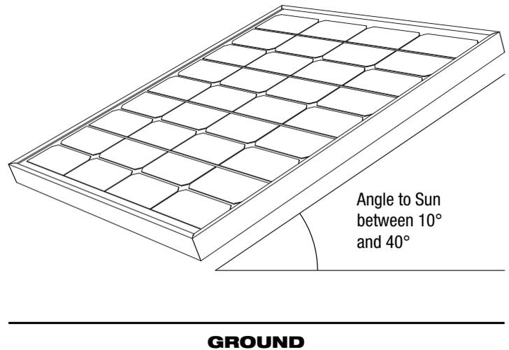
The optimal angle from ground of the panel is around  $30^\circ$ . Anywhere between  $10^\circ$  and  $40^\circ$  ensures good power generation across the course of the day.
